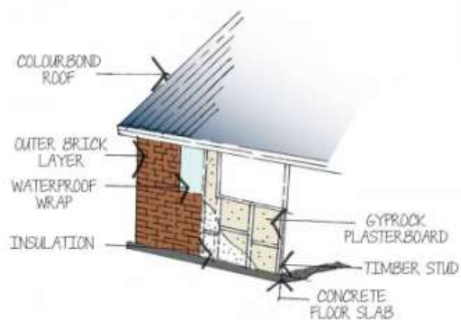
Figure 22: An example of a typical brick veneer construction. This illustration displays an outer brick shell and internal plasterboard lining.
